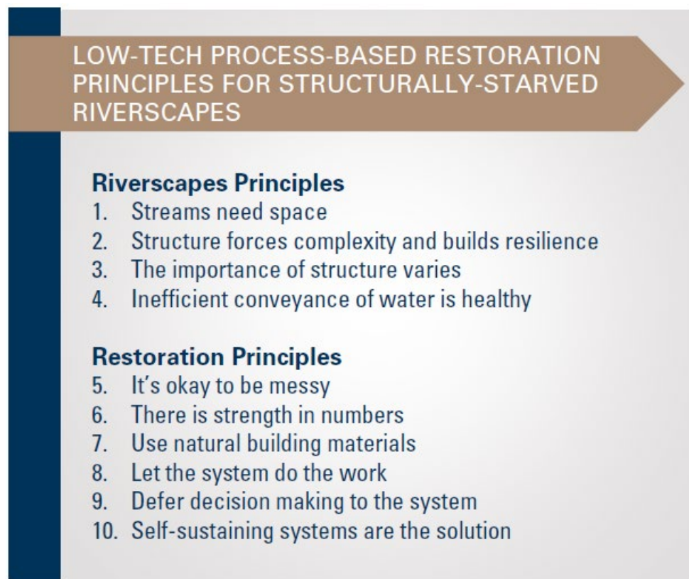
Figure 6. Design Principles for Low-Tech Process Based Restoration Treatments (From Wheaton et al. 2019)
