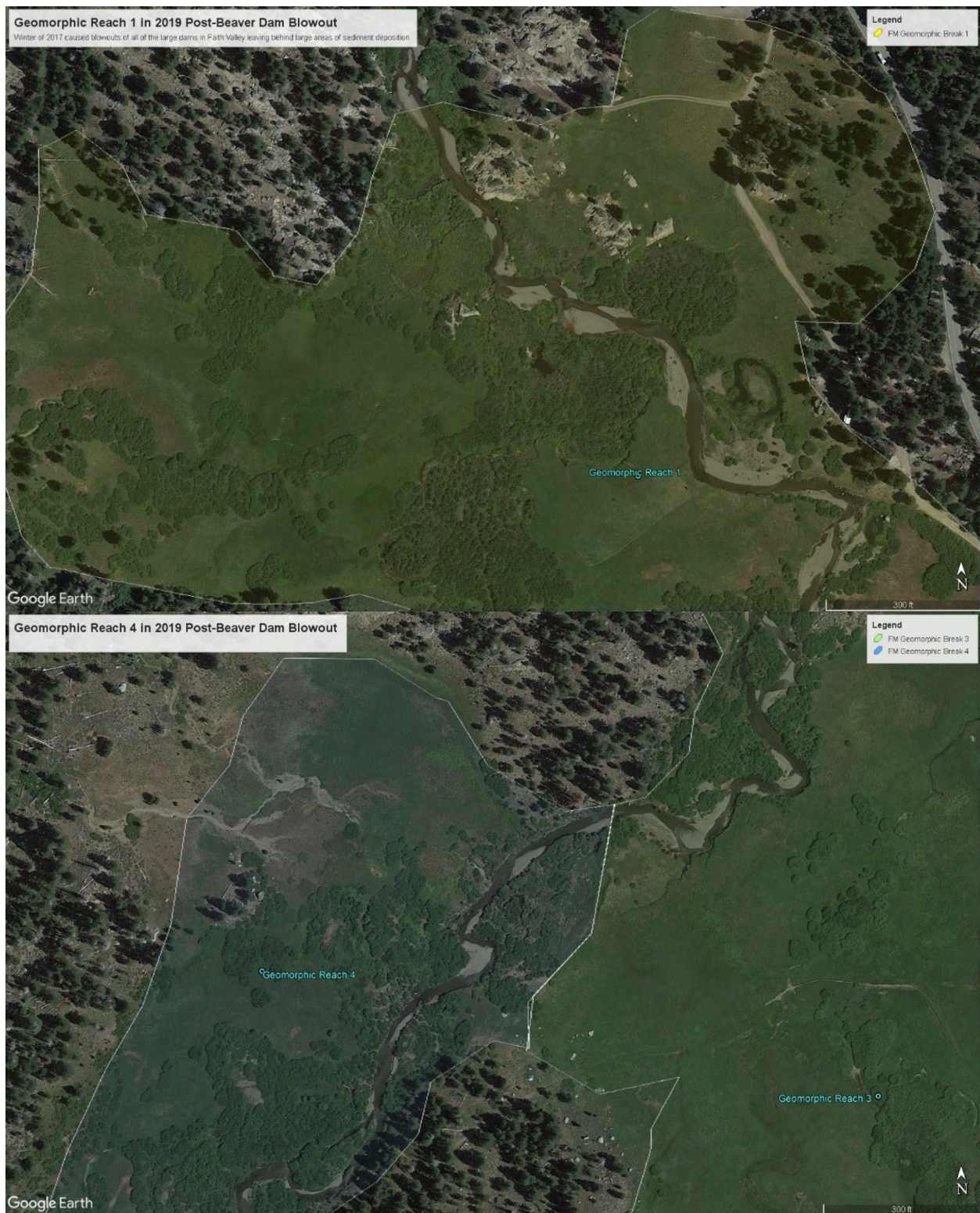
Figure 11. The same reaches as depicted in figure 10 after the heavy flows in 2017 completely breached all of the large beaver dams in Faith Valley. Note the reduction of inundated areas and large areas of fresh sediment deposition exposed and redeposited by the blowout. This is a return to Stage 5-7 in the Stream Evolution Model.
