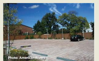
Permeable paving includes a range of materials that allow stormwater to move through a "paved" surface. Permeable pavers can be used in residential or commercial settings and are aesthetically comparable or superior to concrete, asphalt, and other impermeable surfaces.
