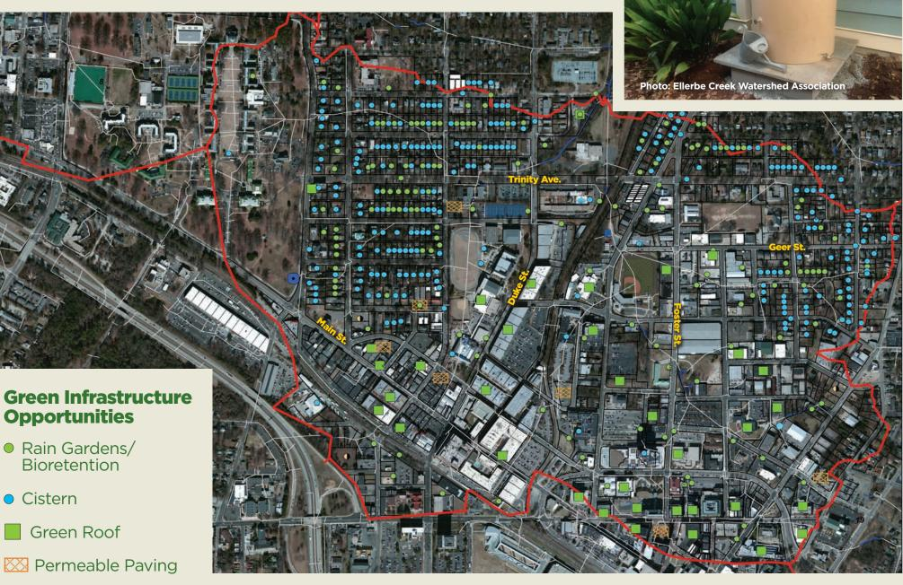
**Cisterns** and other rainwater harvesting devices collect and store rainwater for later use. Rain water can be re-used for watering gardens and yards, washing cars, and other outdoor water needs. Harvesting and using rainwater from a cistern can reduce water bills and reduces the strain on the municipal water system.
