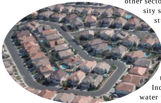
STREETS AND ROOFS CHANNEL WATER INTO STORM DRAINS INSTEAD OF AQUIFERS.
